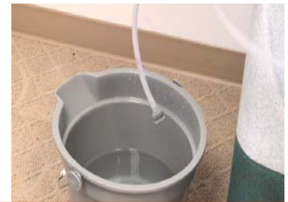
Place Chemical Feed Hose into Rinse Solution
